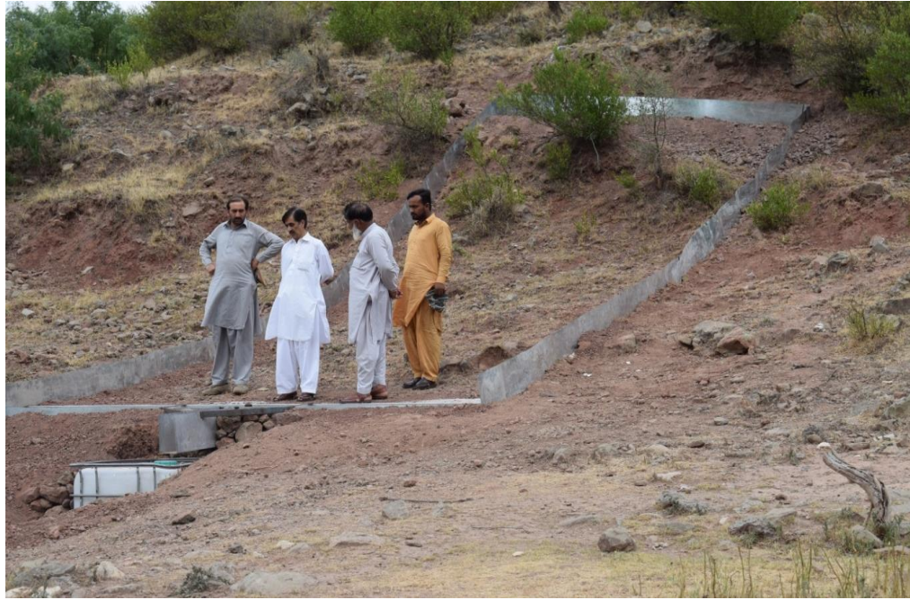
A view of Erosion Plot Established on Barren Land in Samarkand (Chakwal)
